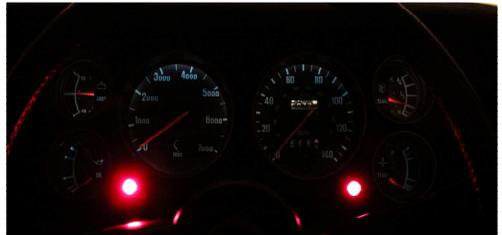
As the bulbs are directly behind the dials, most of the light from the standard 2.2W bulbs gets reflected back behind the instruments and very little makes it way past to be of any use. Therefore I used a 5 SMD LED 360° Ultra White Bulbs from Amazon that have the equivalent of a 10W bulb but with a quarter the power consumption of the 2.2W bulb.
